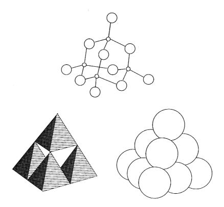
Fig. 2.12 Three expressions for the structure of  $P_4O_{10}$ .
