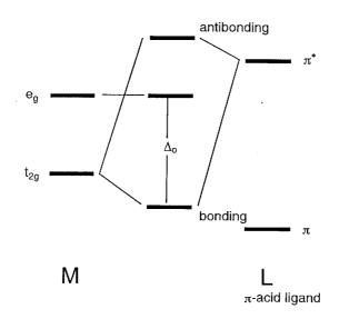
**Fig. 6.12** The energy change upon formation of M-L<sub> $\pi$ </sub> bonds.
