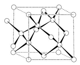
Fig. 4.5 Structure of diamond.
