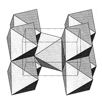
Fig. 4.13 Structure of rutile.
