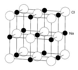
Fig. 2.7 Rock-salt structure.
