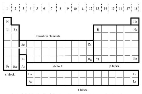
Fig. 1.2 Block classification of elements in the periodic table.
