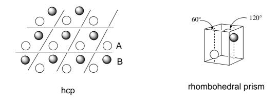
Fig. 2.5 Different expressions of hexagonally close-packed.
