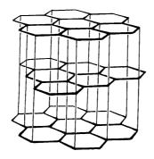
Fig. 4.4 Structure of graphite.
