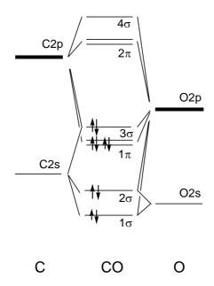
Fig. 2.22 Molecular orbitals of CO.
