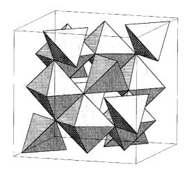
Fig. 4.15 Spinel structure.
