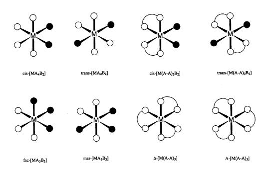
Fig. 6.3 Geometrical isomers of 6-coordination.
